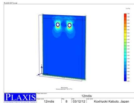
Fig 18: Total strain -twin tunnel with 12m distance
