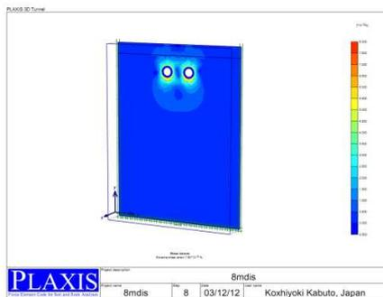
Fig 14: Total stress with tunnel with 8m distance
