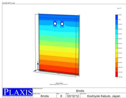
Fig 13: Total strain twin tunnel with 8m distance
