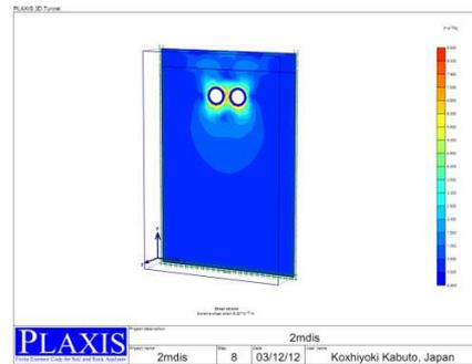
**Fig12: Total strain - twin tunnel with 2m distance**
